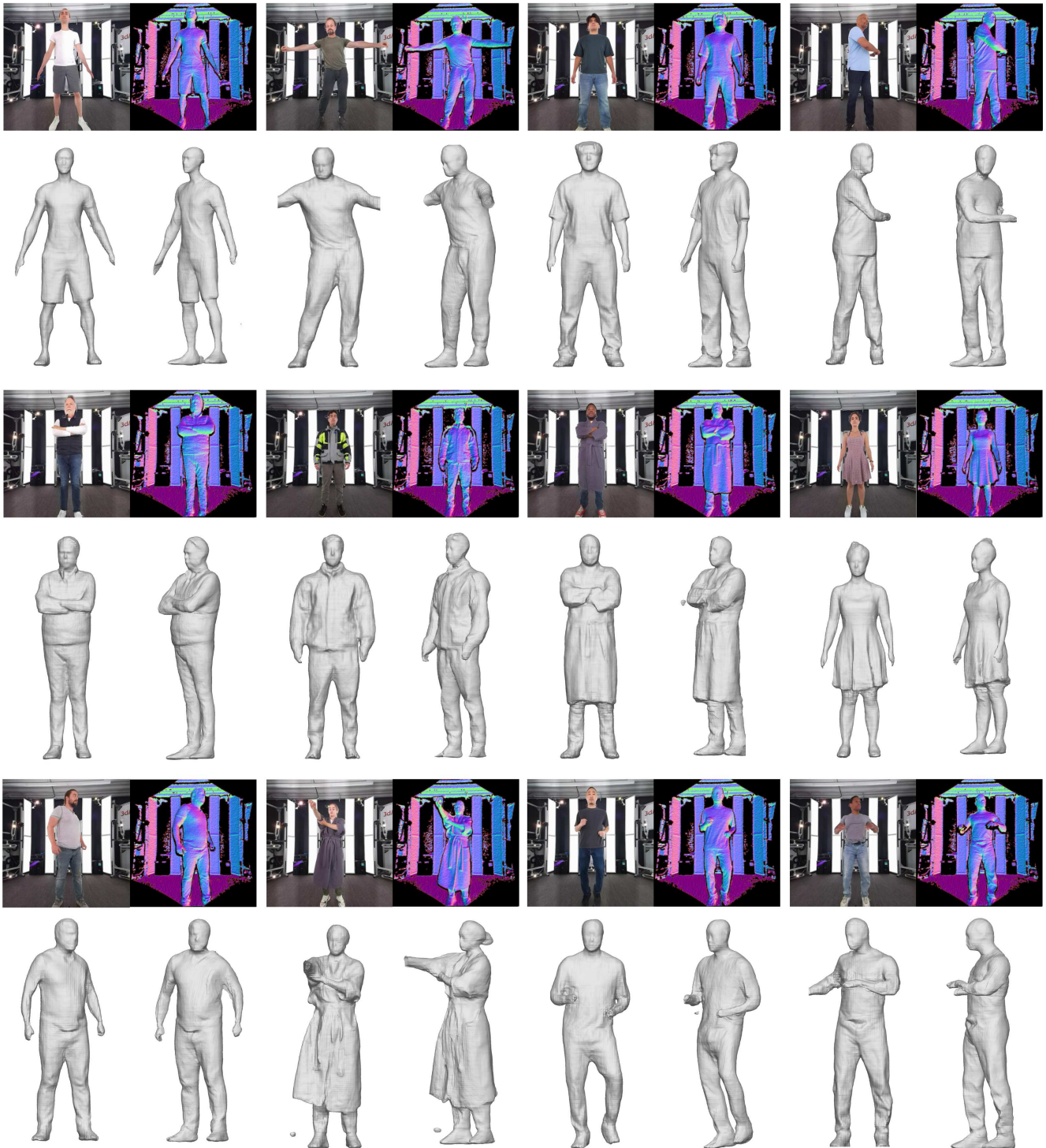
Figure 10. More reconstruction results by ANIM using a consumer-grade RGB-D camera (Azure Kinect) as an input. ANIM is capable of handling various human body and cloth typologies ranging from a skirt to a bath robe and is agnostic to diverse human poses.
