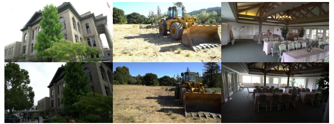
Figure SB.1. Inconsistent camera exposure problem on TnT. Each image was captured with a different and unknown camera exposure. This misleads photometric optimization methods that assume pixel color consistency across stereo views to triangulate 3D points, including 2DGS and our PAGaS.
